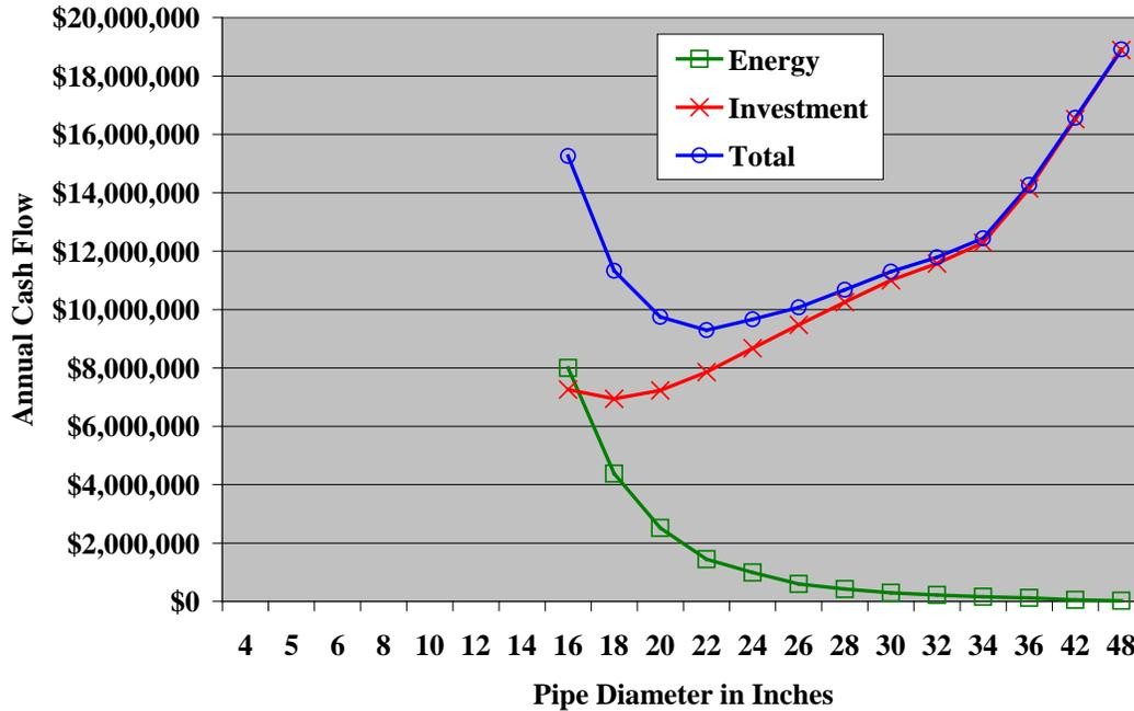
**Graph 16. Optimized Pipe Diameter for 13,000 GPM and 50,000 Feet Distance**
