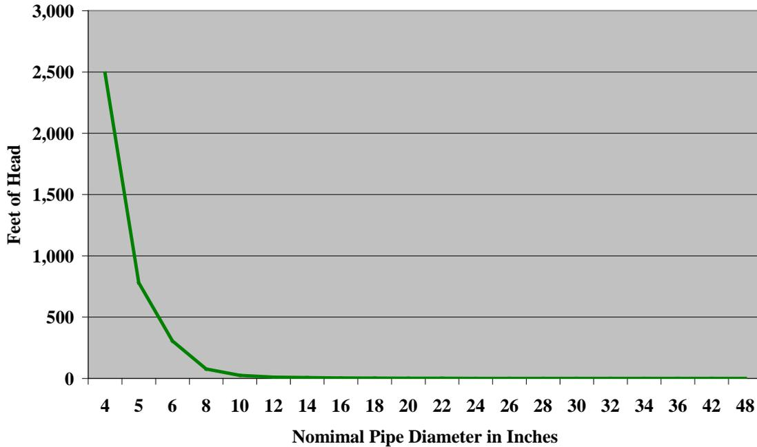
**Graph 2. Head Loss as a Function of Pipe Diameter**
