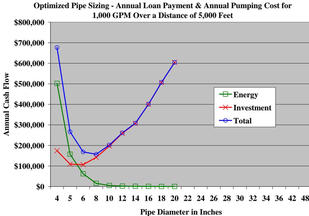
**Graph 7. Optimized Pipe Pump Sizing for 1,000 GPM**
