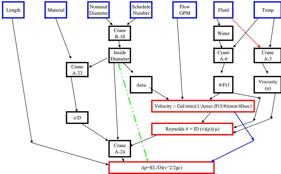
**Figure 1. Flow Charting the Pressure Drop Equations**
