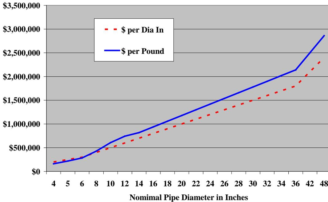
**Graph 3. Installed Pipe Cost as a Function of Diameter**
