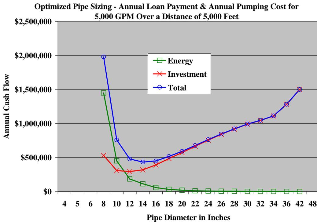
**Graph 8. Optimized Pipe Pump Sizing for 5,000 GPM**
