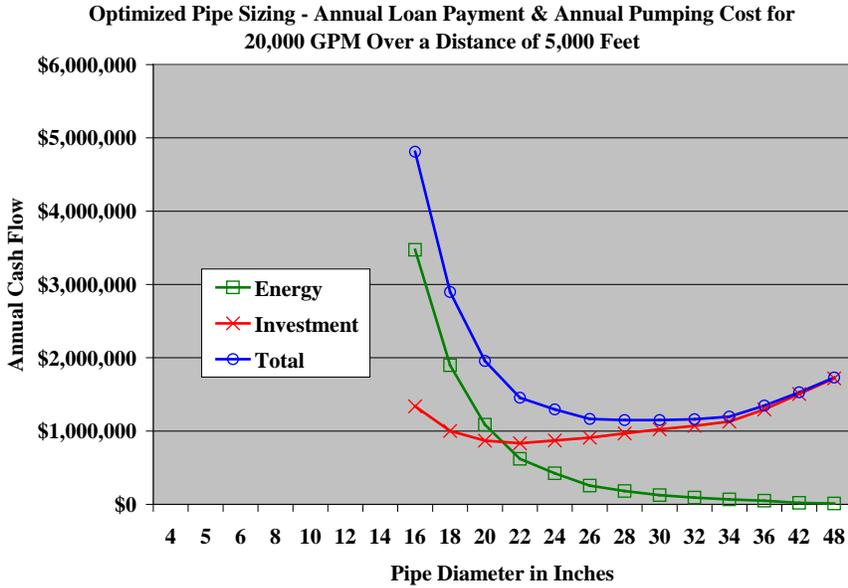
**Graph 11. Optimized Pipe Pump Sizing for 20,000 GPM**
