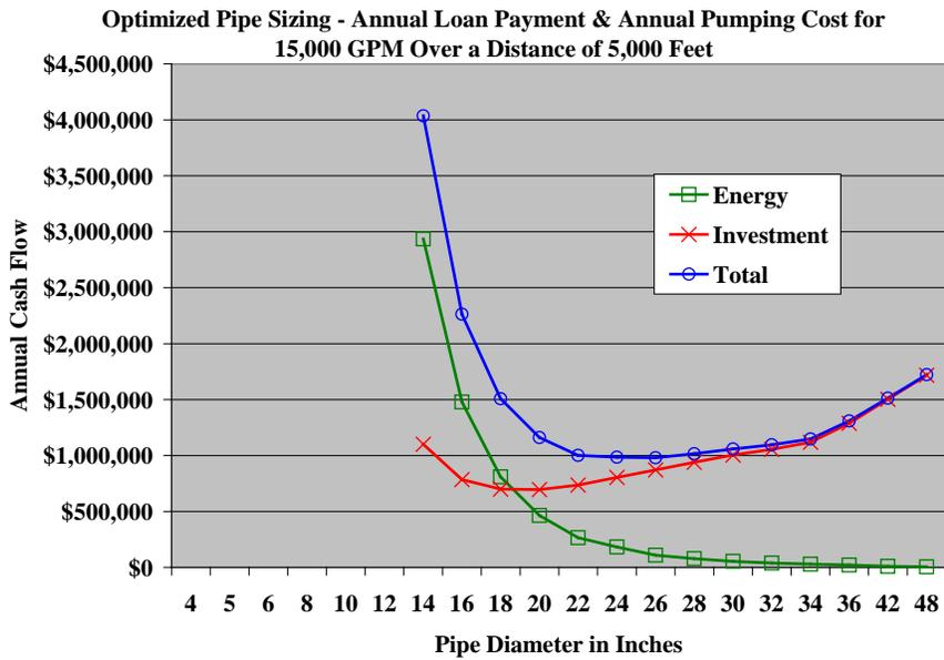
**Graph 10. Optimized Pipe Pump Sizing for 15,000 GPM**
